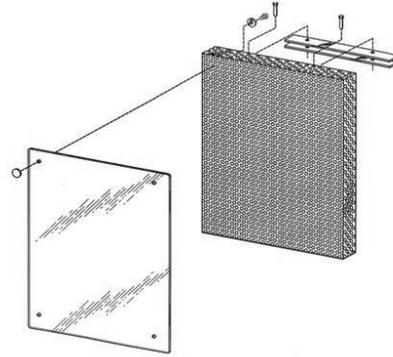
The **Agency Version** has a single layer of acrylic that presses the media being framed directly against the metal frame. All **architek** frames come with a unique architectural hanging system.
